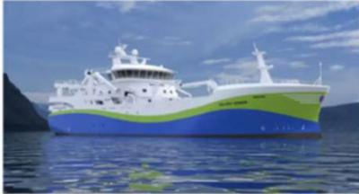
This 70m Norwegian longliner will have two 185-kW hydrogen fuel cells and a 2,000-kWh battery bank, as well as conventional diesel engines.
