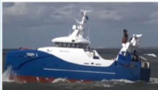
The special shape of the ship and the diesel electric propulsion provide 60% fuel and CO<sub>2</sub> savings compared to comparable fishing vessels.
