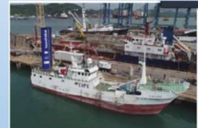
Balueiro Segundo with eSAIL® system, co-funded via EU Aspiring Wingsails project
